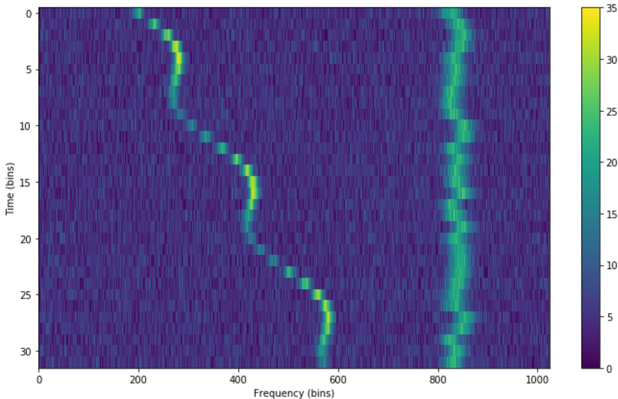
`setigen` is a Python library for generating and injecting artificial narrow-band signals into radio frequency data. `setigen` interfaces primarily with two types of data: spectrograms or dynamic spectra, saved in two-dimensional NumPy arrays or filterbank files (.fil extension), and raw voltages (GUPPI RAW files). Both data formats are instrumental to Breakthrough Listen’s data collection and analysis pipelines.
