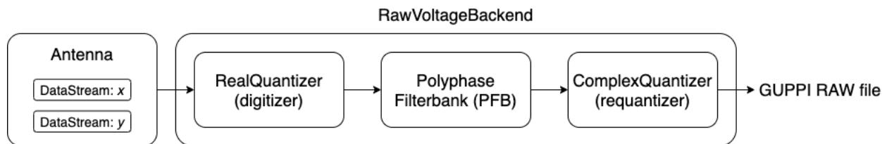
The basic layout of a voltage pipeline written using `setigen.voltage` is shown in the image.
